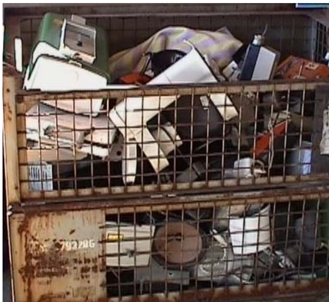
Figure 67: Collection of waste electrical and electronic equipment in a waste material collection centre, fraction small electrical and electronic appliances
