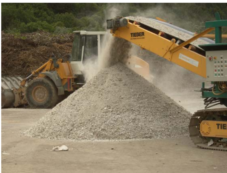
Figure 76: Generation of a gypsum raw fraction from gypsum plaster boards; experiment performed in the context of the project "Gipskartonplatten-Recycling".
