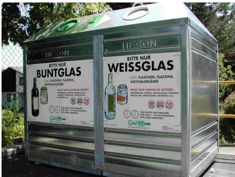
Figure 52: Double chamber container for waste glass collection, lifting system
